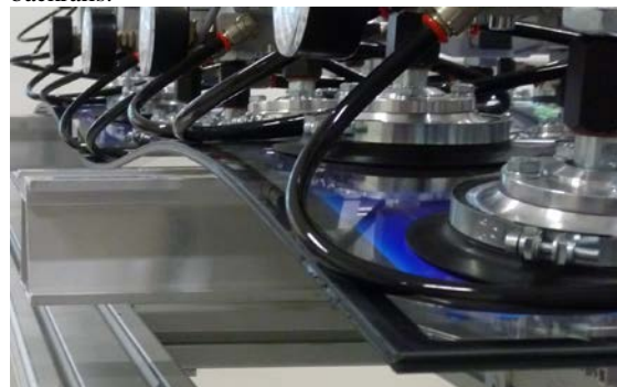
Figure 11: “TPedge”-module with 2 mm glass panes, backrails and supported mounting during mechanical load test (2400 Pa)
