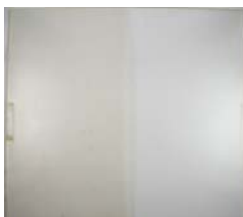
Figure 1: Glass sample after 2 years exposure at Negev Desert, Israel
