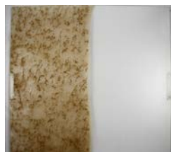
Figure 2: Glass sample after 2 years exposure at Canary Island, Spain
