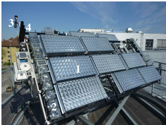
Figure 1: Modules and equipment of the SOPHIA module round robin mounted on the sun tracking unit at Fraunhofer ISE in Freiburg: (1) SOITEC MX400 modules (2) SOITEC-ISE mono-module (3) pyrheliometer (4) component cell sensor
