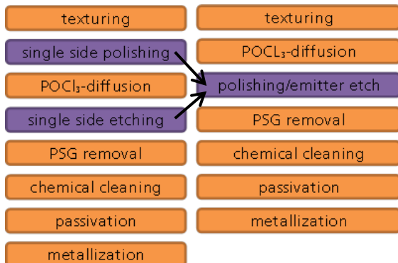
Figure 1: Process scheme for the PERC solar cell concept with the standard process (left) and combined wet chemical process (right). The orange highlighted steps are two side processes and the purple highlighted are single sided process steps.
