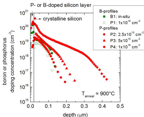
**Figure 4:** Boron (B) and phosphorus (P) doping profiles in the silicon layer and in crystalline silicon obtained by ion implantation at different doses and after annealing at 900°C. The first data points correspond to measurements of the B- and P-doped silicon layer which are prone to errors. The vertical line represents the approximate position of the interface.
