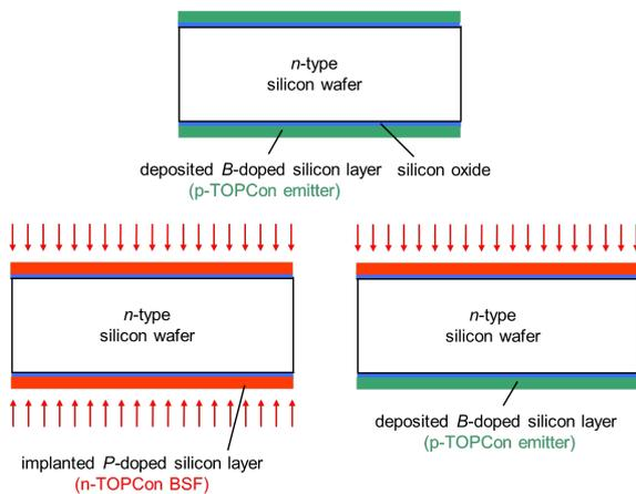
**Figure 2:** Schematic illustration of the lifetime (bottom, left) and Suns- $V_{oc}$  samples (bottom, right) that were fabricated by ion implanting a phosphorus doping into an in-situ boron-doped TOPCon emitter (top) to overcompensate the emitter and obtain a phosphorus-doped TOPCon BSF (bottom).
