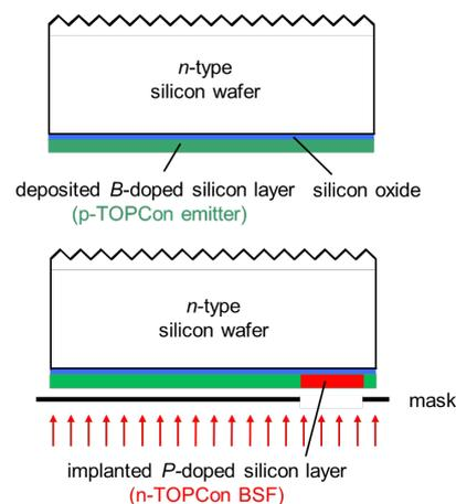
**Figure 1:** Schematic illustration of the interdigitated back contact (IBC) silicon solar cell with a tunnel oxide passivated contact (TOPCon) where the in-situ boron-doped TOPCon emitter (top) is locally overcompensated by ion implanted phosphorus using a mask to obtain a phosphorus-doped TOPCon BSF (bottom).
