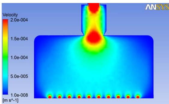
Fig. 2: Velocity profile of a parallel dispensing print head, as described in [7]: After investigating several nozzle types using this CFD-model concerning flow rate and pressure distribution, hardware design was expanded towards a multi nozzle application. Here, investigations were focusing on a homogeneous paste flow distribution within the print head with as little pressure drop as possible.
