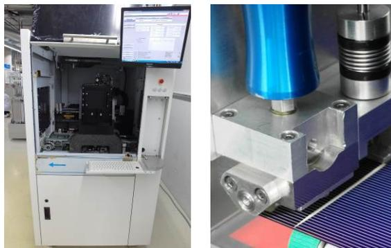
Fig. 3: Completely new developed, inline applicable dispensing platform at Fraunhofer ISE's PV-TEC (left) with integrated advanced version of the ten nozzle print head (right) during cell manufacturing.
