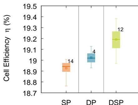
Fig. 6: Cell efficiencies on 156x156mm<sup>2</sup> Cz-p-type material with industrial high ohmic emitters. Single screen printing (SP) is compared with double screen printed (DP) and dispensed (DSP) technology.
