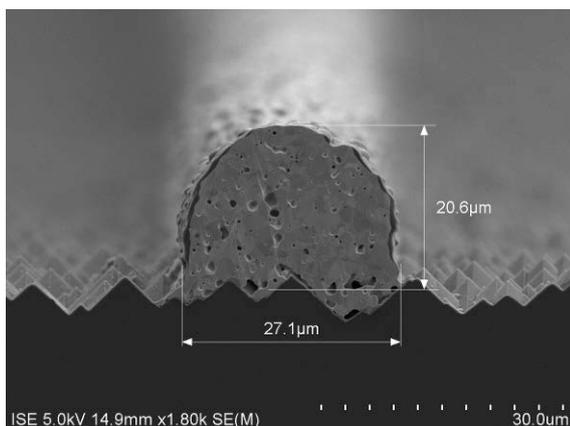
Fig. 1: Finger cross section of dispensed contact fingers using a new developed screen printing paste (top) and a dispensing paste with adapted rheology (bottom, from [2]), both printed in a parallel dispensing unit with a nozzle opening of just 40µm.
