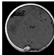
**Figure 7:** SAM image of a bond between a 2" GaSb wafer and a 4" GaAs wafer with a metamorphic buffer and a  $\text{Ga}_{0.79}\text{In}_{0.21}\text{As}$  bond layer. Only the 2" GaSb wafer is visible. Black areas arise from rough backside of the GaSb wafer.
