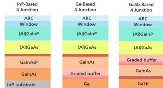
**Figure 1:** Different cell architectures for wafer-bonded 4-junction solar cells. The bond position is always indicated by the red line. Left: InP-based concept with wafer-bond between (Al)GaAs- and GaInAsP-junction. Center: Ge-based concept with wafer-bond between (Al)GaAs- and GaInAs-junction. The GaInAs junction is obtained by metamorphic growth on the Ge substrate. Right: GaSb-based concept with wafer-bond between GaInAs- and GaSb-junction.
