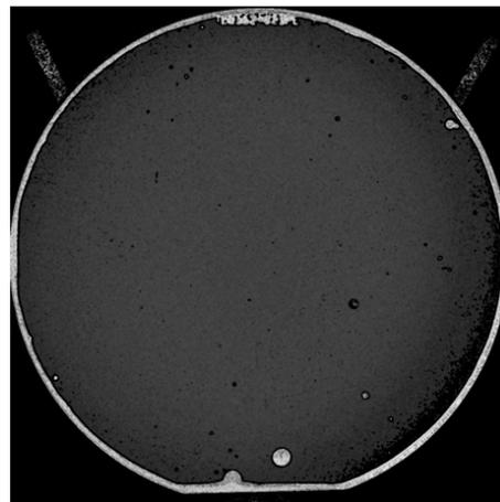
**Figure 2:** Scanning Acoustic Microscope (SAM) image of a bonded structure of a 4" GaAs wafer and a 4" Ge wafer with a metamorphic buffer on top. Bonded areas are black, non-bonded white. The wafers are completely bonded, except for some small bubbles. The wafer laser marking can be seen on top of the bond.
