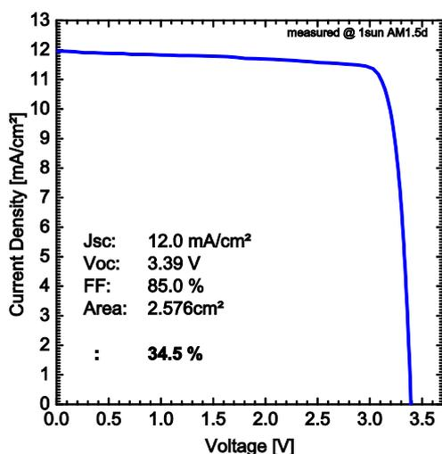
**Figure 5:** I-V characteristics of cell 2, a bonded 4-junction cell on Ge. An efficiency of 34.5% was measured under one sun AM1.5d illumination.
