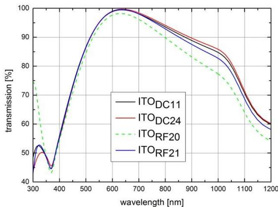
**Figure 3:** Transmission curves for different magnetron sputtered ITO films on glass
