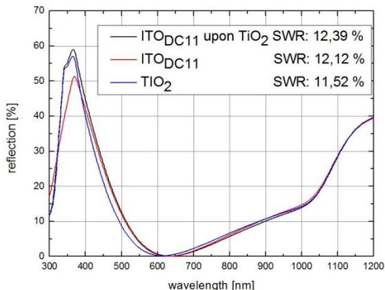
**Figure 7:** Reflection for an ITO<sub>DC11</sub>/TiO<sub>2</sub> stack in comparison to the corresponding single layers
