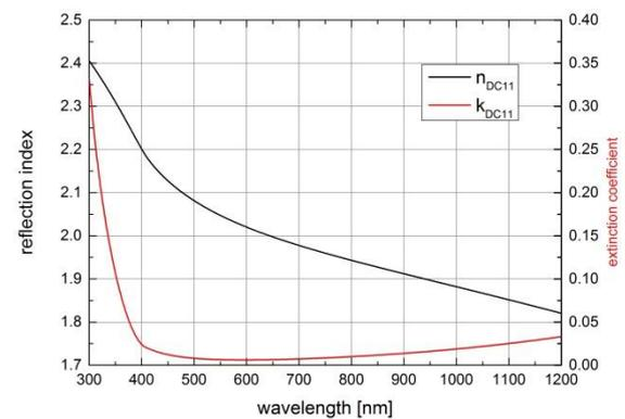
**Figure 1:** Optical constants for ITO film DC11 determined from spectroscopic ellipsometry measurement
