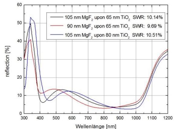
**Figure 5:** Reflection curves for MgF<sub>2</sub>/TiO<sub>2</sub> stacks with different MgF<sub>2</sub> thicknesses
