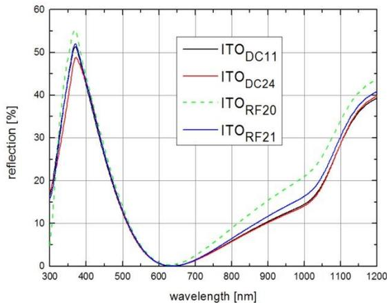
**Figure 2:** Reflection curves for different magnetron sputtered ITO films on silicon
