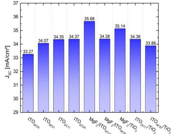
**Figure 8:** Calculated  $J_{sc}$  for different simulated ARCs
