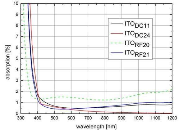
**Figure 4:** Absorption curves for different magnetron sputtered ITOs
