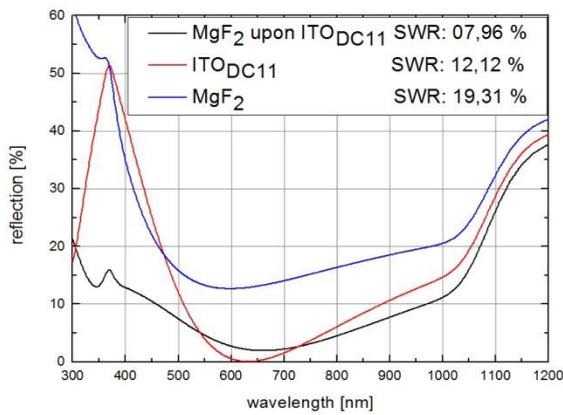
**Figure 6:** Reflection curve for an MgF<sub>2</sub>/ITO<sub>DC11</sub> stack in comparison to the corresponding single layers
