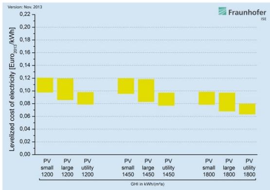
Figure 2: LCOE of various PV plant types at three locations with high solar irradiation (GHI in kWh/(m 2 a)) in 2013, (Fraunhofer ISE, 2013).
