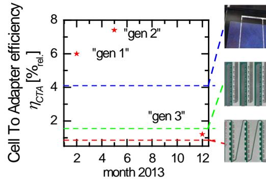
Figure 7: Evolution of the relative efficiency CTA-losses for the submodules generations 1-3. The red stars represent the achieved CTA efficiency on submodule level within the project. The continuous lines display the calculated CTA efficiency losses based on analytical and numerical calculations.
