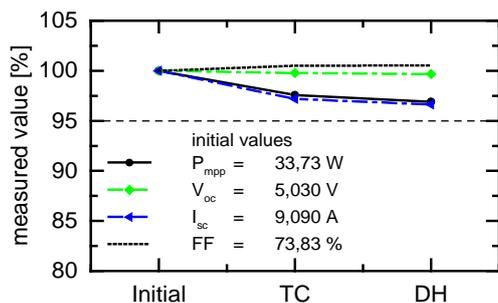
Figure 10: IV characteristics of module B before after reliability testing sequences
