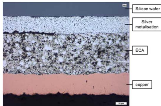
Figure 9: Cross section image of a TPU-adapter/conductive epoxy/cell contact (500x magnification) showing void
