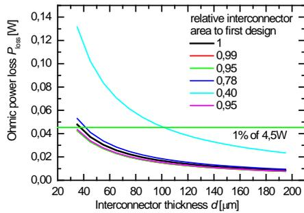
Figure 3: Simulated absolute power loss in watt for different circuit designs as a function of the copper thickness. The targeted power loss of 1%<sub>rel</sub> is indicated by the green line.
