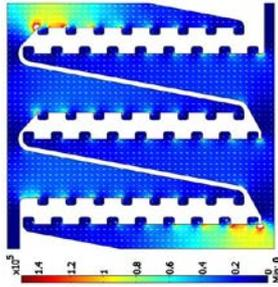
Figure 2: FEM analysis of the structured copper layer in 75µm thickness of the TPU-adapter: ohmic loss in W/m³
