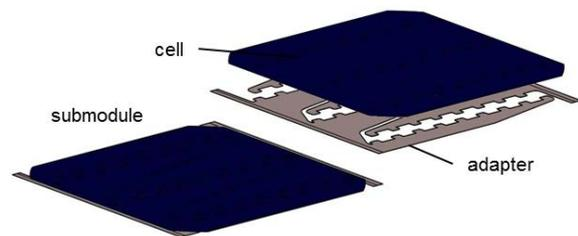
Figure 1: Module integration concept for back-contact solar cell. The cell is laminated on an interconnection adapter based on a polymer sheet and a copper circuitry.
