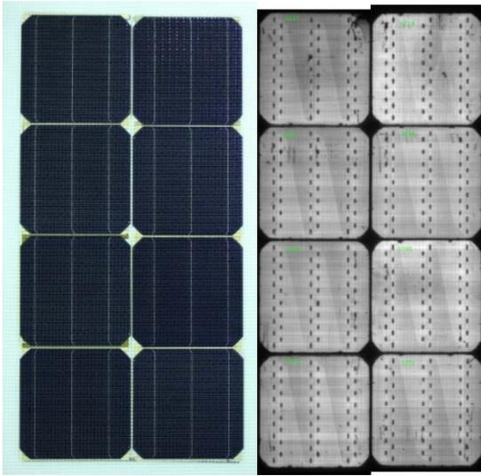
Figure 6: Photograph (left) and electroluminescence image(right) of module A
