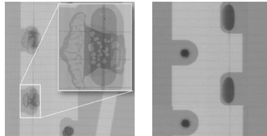
Figure 8 a) (left): Radiographic x-ray image of interconnection joints of a submodule of the first generation (gen 1) showing incomplete coverage of the contact pads with conductive adhesives and void formation. b) (right): showing optimized conductive adhesive joint without voids and with optimal coverage of contact pads.
