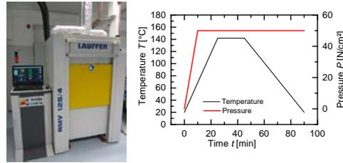
Figure 4: PCB Lamination Press used for submodule assembly Figure 5 Lamination Profile of temperature and pressure during submodule lamination
