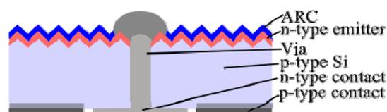
**Figure 1:** Schematic cross section of a p-type silicon MWT-BSF+ solar cell without rear emitter resulting from the process sequence shown in Figure 2. The rear emitter is removed by a single-side emitter etch back, which most likely also removes the emitter in the vias.
