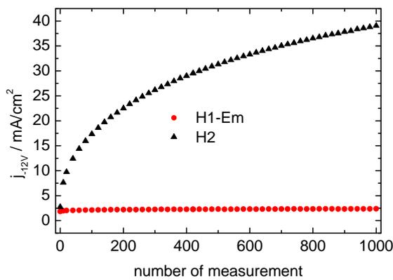
**Figure 10:** Current densities  $j_{-12V}$  measured at a reverse bias of  $V = -12$  V of repeated *I-V* measurements of one representative cell per group H1-Em and H2 after degradation. The cells were measured 1000 times under reverse and forward bias. For reasons of clarity only each 20<sup>th</sup> measurement is presented. Group H1 exceeded  $j_{-12V} = 45$  mA/cm<sup>2</sup> throughout the experiment.
