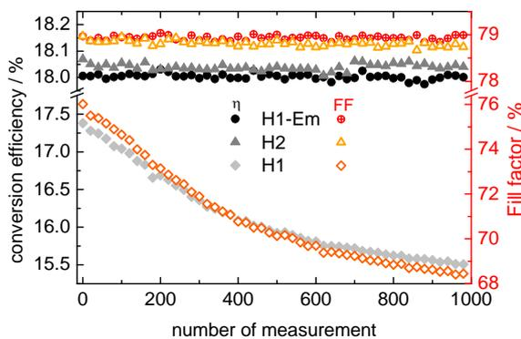
**Figure 11:** Conversion efficiencies  $\eta$  (filled markers) and fill factors  $FF$  (hollow markers) of repeated *I-V* measurements of one representative cell of each group after degradation. For reasons of clarity only each 20<sup>th</sup> measurement is presented.
