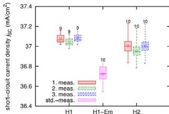
**Figure 3:** Short-circuit current density  $j_{SC}$  of the fabricated MWT-BSF cells according to the  $I$ - $V$  measurement sequence shown in Table I. The whisker reaches from minimum to maximum, the box is from the lower to the upper quartile, the horizontal line indicates the median and the square the average. The number above the whisker states the number of measured cells.
