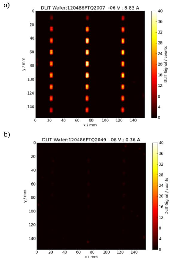
Figure 9: DLIT images for MWT-BSF solar cells with via pastes (a) H1 and (b) H2 printed directly on the p-type silicon base.
