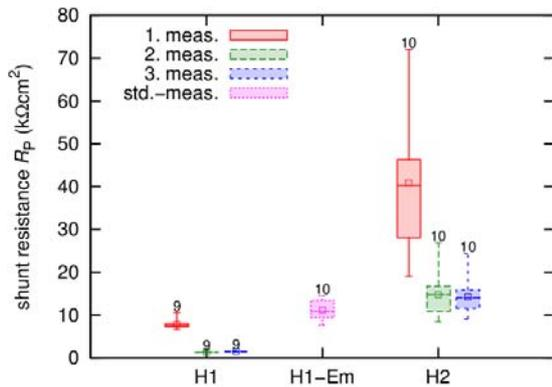
Figure 6: Shunt resistances  $R_p$ .
