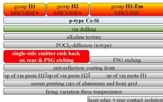
**Figure 2:** Process sequence for fabrication of p-type MWT-BSF solar cells without (left) and with rear emitter (right). The process sequence for MWT-BSF solar cells without rear emitter consists of one process step less than the process for MWT-BSF cells with rear emitter as the emitter etch back and the PSG etch are realized in one process step.
