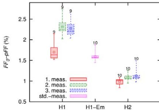
Figure 7: Difference between ideal fill factor ( $FF_0$ ) and series resistance-independent pseudo fill factor ( $pFF$ )  $FF_0 - pFF$ .
