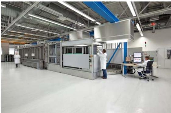
**Figure 4:** ProConCVD at SIMTEC laboratory of Fraunhofer ISE
