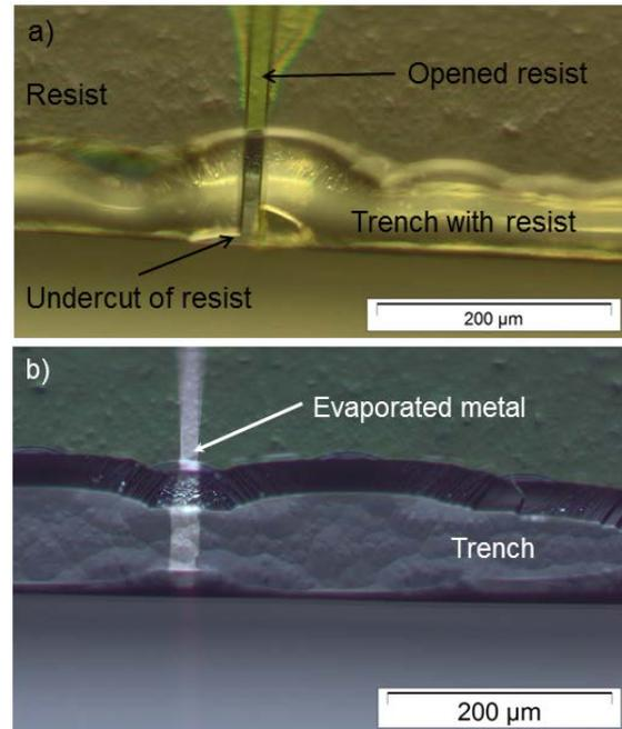
**Fig. 6:** Microscopy image of tilted sample with etched trenches, view perpendicular to the flank of a trench. a) Sample with negative photoresist after exposure and development. b) Sample after evaporation of metal and lift-off of resist.
