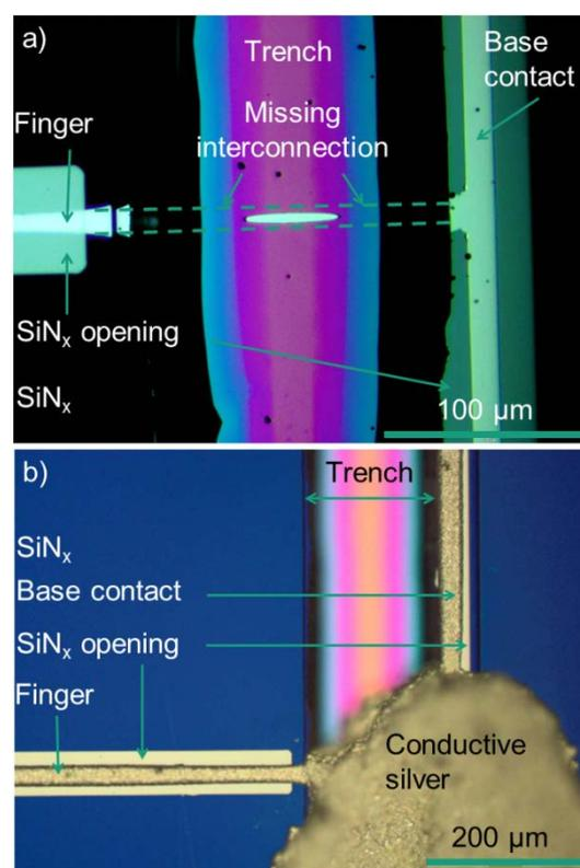
**Fig. 4:** Interconnection between two neighboring cell strips. Emitter contact is running from the left over the trench to connect to base contact of the next cell on the right. a) Interconnection in the trench is missing. b) Interconnection established by conductive silver, afterwards electro-plating is possible.
