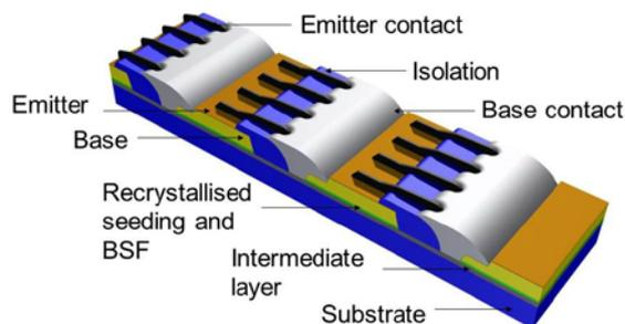
**Fig. 1:** Detail of integrated interconnected module with screen-printing interconnection (not to scale).
