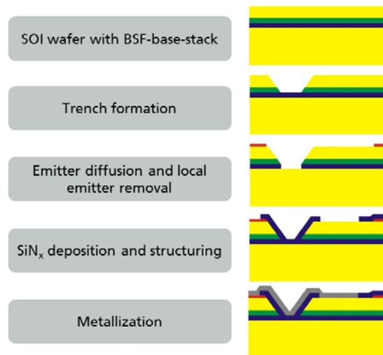
**Fig. 2:** Sequence of laboratory process to form integrated interconnected crystalline silicon thin-film modules. The process starts with the substrate (yellow) with  $\text{SiO}_2$  intermediate layer (blue), back surface field (BSF) (green) and base (yellow) on top. The emitter is displayed in red, the  $\text{SiN}_x$  isolating layer in blue and the metallization is grey.
