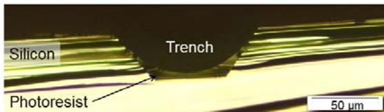
**Fig. 5:** Microscopy image of cross section of sample with etched trenches after spin-coating of photoresist.
