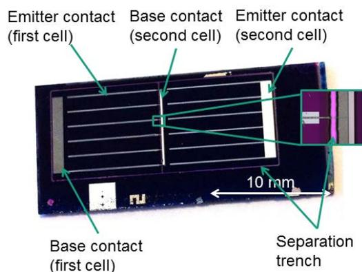
**Fig. 3:** Mini-module consisting of two cells with 10 mm cell width each.
