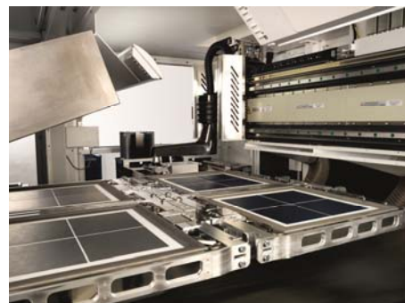
Figure 2: View into the wafer loading/unloading unit of the VCS1200 including wafers which are placed on deposition carriers.
