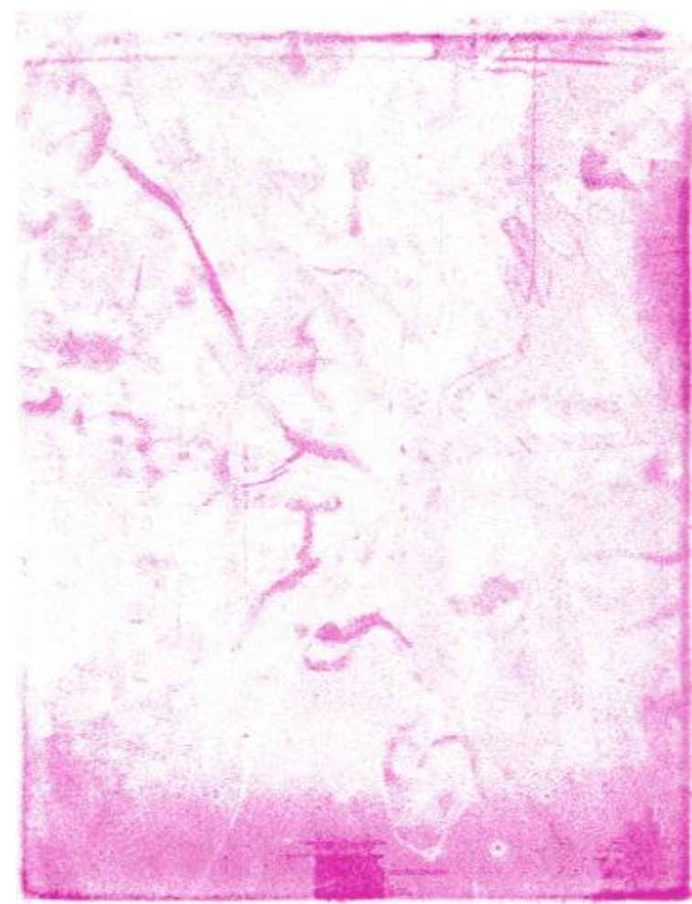
Max. pressure distribution on compressed pouch cell surface without cushioning foam (0.05 - 2 MPa)
