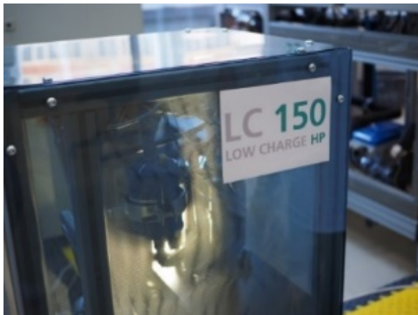
The heat pump with the climate-friendly refrigerant propane from the "LC150" project. © Fraunhofer ISE
