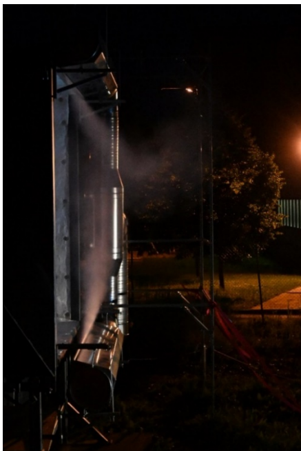
The airflow separates the hot inside of the receiver (left) from the outside air. © Fraunhofer ISE
