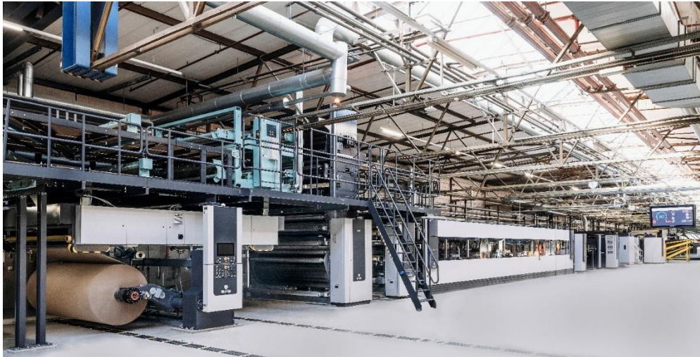
The so-called "wet end" of a corrugator from BHS Corrugated. © BHS Corrugated
