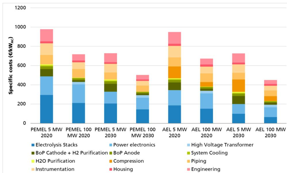
Figure 2: Alkaline and PEM electrolysis system cost for different system capacities in 2020 and 2030. ©Fraunhofer ISE
