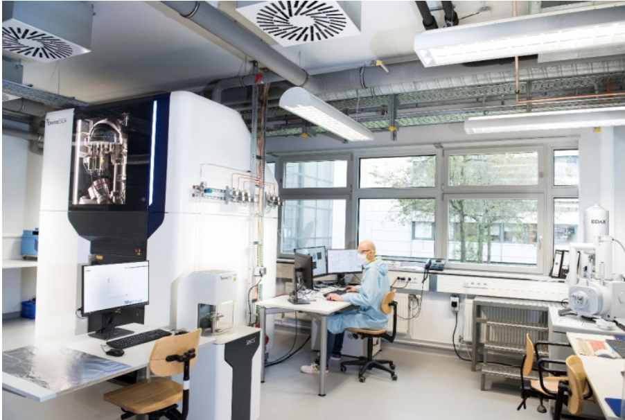
The X-ray Photoelectron Spectroscopy device EnviroESCA in the laboratory of Fraunhofer ISE in Freiburg, Germany.
