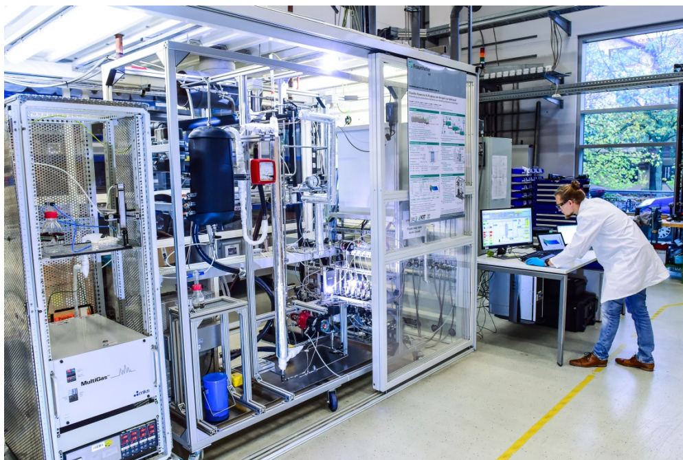
Scale-Down-Miniplant zur Erforschung der Methanolsynthese am Fraunhofer ISE. © Fraunhofer ISE
