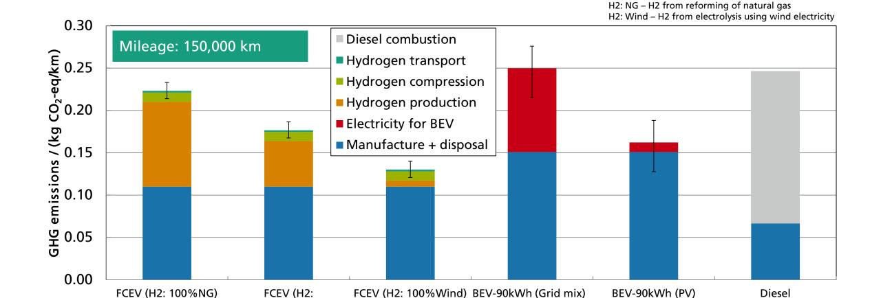
Diesel combustion also includes GHG emissions for diesel supply
