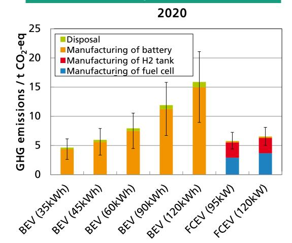
GHG fuel cell system (95 kW) ≈ GHG battery with 60 kWh
