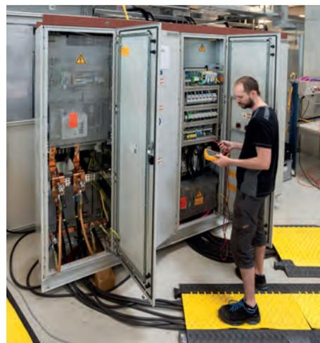
1 MW Batterie-simulator im TestLab Power Electronics.
