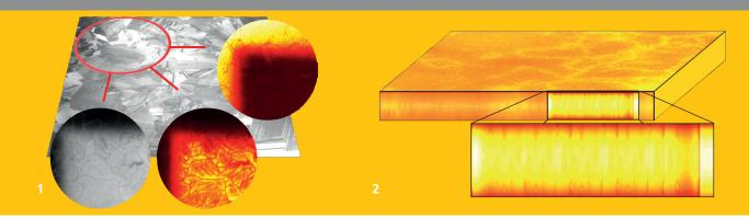
Photoluminescence based defect imaging of a multicrystalline wafer (left to right: photoluminescence of an as-cut wafer, lifetime map, interstitial iron concentration).
