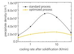
4 Overall density of iron precipitates in dependence on the cooling rate after solidification and the phosphorus diffusion process.
