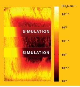
simulations enables us to predict the distribution of impurities after optional process variations. The experimentally confirmed simulation results can then be used as input parameter for simulations concerning the optimization of the impurity distribution.
