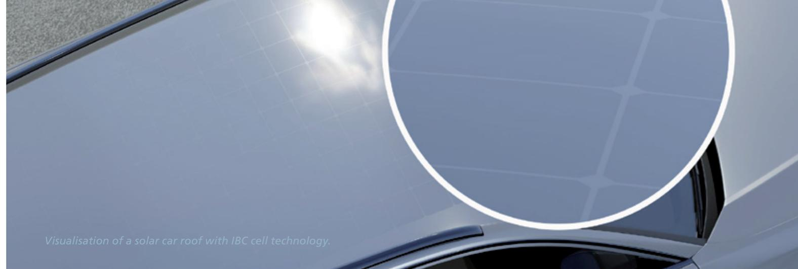
Visualisation of a solar car roof with IBC cell technology.
