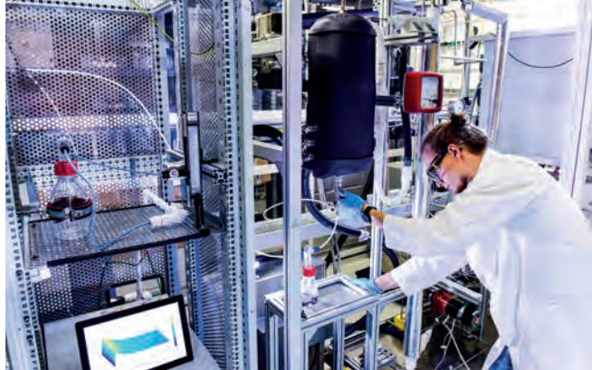
Mini plant for developing industrial scale methanol synthesis.
