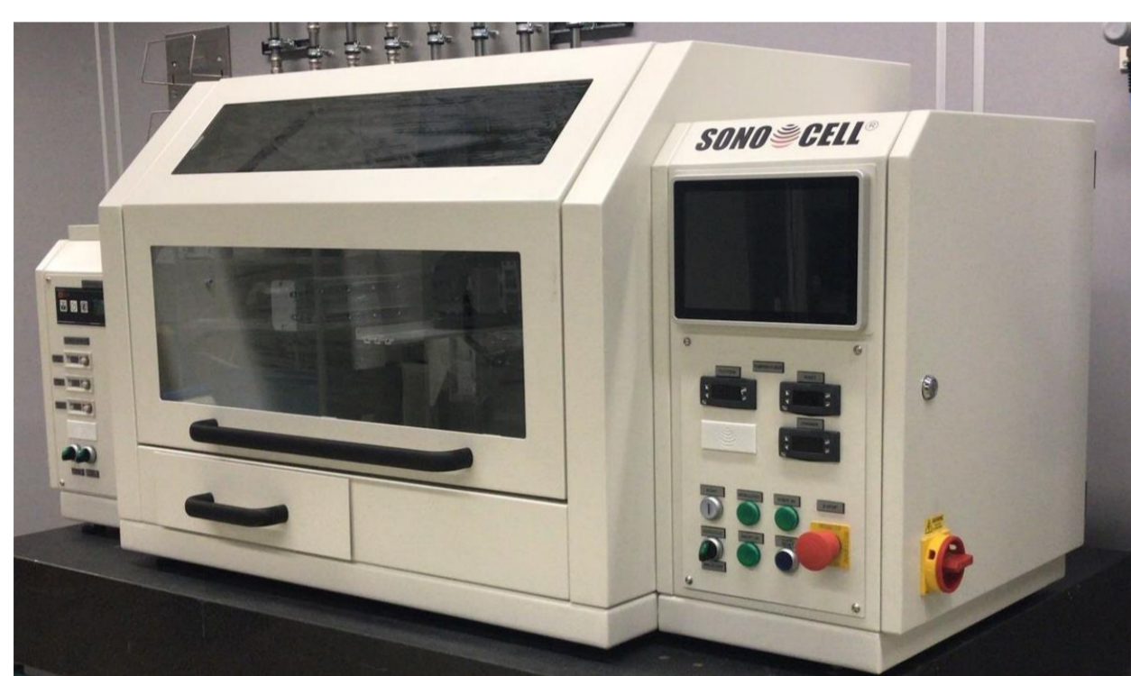
Left: Custom table top spray coater by the company Eqiosonics
