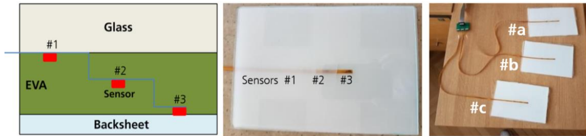
Figure 1 Schematic representation of the sensors positions in the laminate. Middle: Overview of the components used for assembling the laminates before adding the backsheet. Right: Assembled samples after lamination with an external digital acquisition reader
