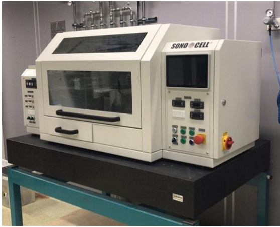
Figure 1: Laboratory spray coating / pyrolysis tool at Fraunhofer ISE
