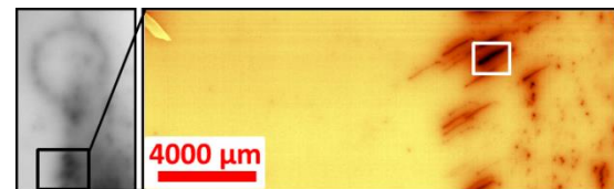
Figure 11: PL image of defective handled area. Marked position is analyzed by \mu -PL (left). \mu -PL image of defective handled area with marked area further investigated by SEM (Figure 12) and EDX (Figure 13) (right).
